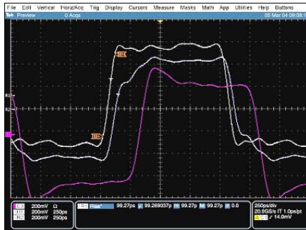
Solder-in Adapter w/ Damping R's
