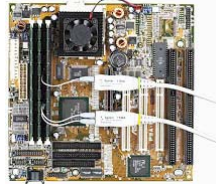
Probing in confined spaces
